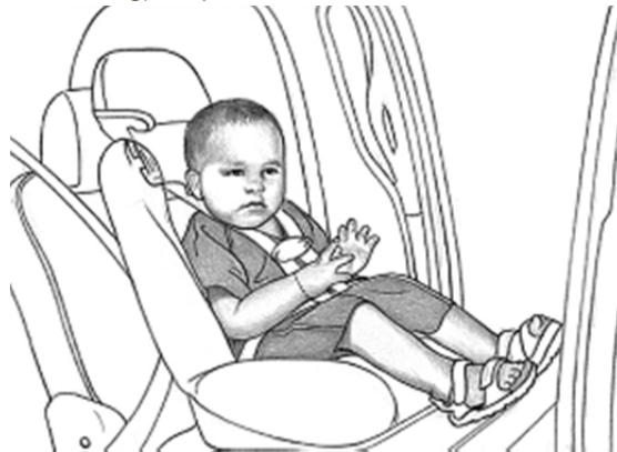
Figure 2: Forward-facing car safety seat
