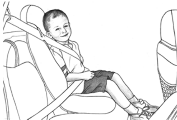
Figure 3: Belt-positioning booster seat
